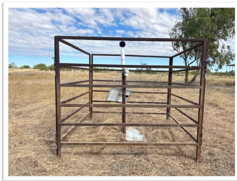
Figure 1 - Noise Monitoring Device
