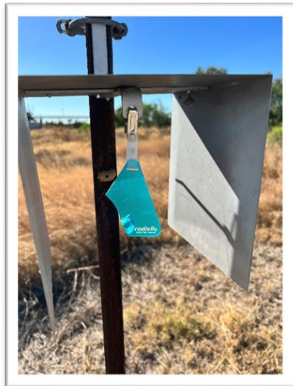
Figure 13 - Radiello Rat Damage (May 2024)
