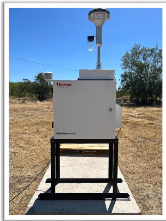
Figure 1 - Partisol 2500i Dichotomous Sequential Air Sampler
