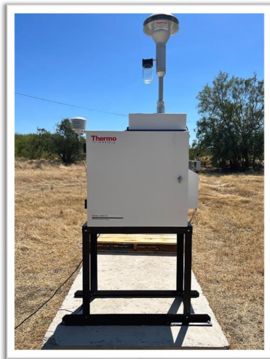
Figure 1 - Partisol 2500i Dichotomous Sequential Air Sampler
