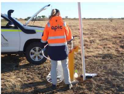
Figure 3. Sampling a groundwater monitoring bore
